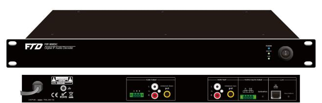
The IP public address system network audio Pre-Amplifier with decoder is the main equipment of the IP network PA system. It is built-in decoder which can decode the network audio signal into analog to feed in analog amplifier.
